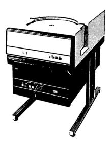
2260 TEN MEGABYT FIXED/REMOVABLE DISK DRIVE Disk Latency Time — Once it is positioned over the appropriate track, the read/write head must wait for the desired sector in that track to rotate to its position. This wait is called the disk latency period. Since the platter makes one complete revolution in 25 milliseconds, the average latency time is one-half this time, or 12.5 ms (.0125 sec).
