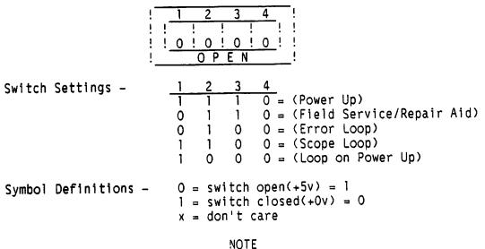
If the controller is not responding properly, it is necessary to run Power Up tests. For more information look under <u>2200 Kennedy Tape Power Up Diagnostic</u> Documentation (760-1102).
