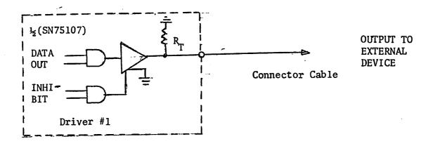
This single connecting wire system is adequate for short lines up to 100 feet where environmental noise is not severe.
