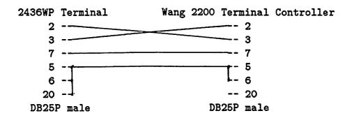
Connect one end of the cable (possibly labeled 'MUX') to one of the four ports on the Wang 2200 terminal controller (2236MXD or 2236MXE). Make sure this port has the correct baud rate setting.
