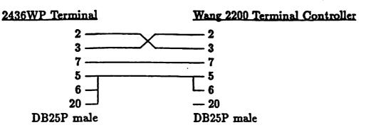
NOTE: Cable lengths over 50 feet may require high quality cable or a reduced baud rate for proper operation.
