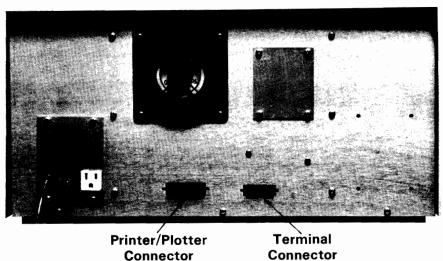
Figure 2-1. 2200SVP Peripheral Connectors
