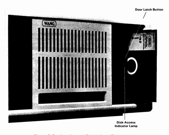
Figure 3-2. Loading and Removing a Diskette
