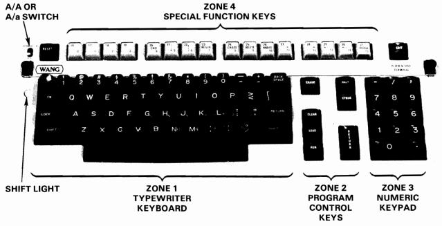
Figure 2-3. Model 2236DE Interactive Terminal Keyboard
