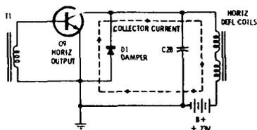
FIGURE 5-11 HORIZONTAL OUTPUT
