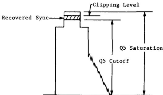
FIGURE 5-5 - SYNC SEPARATOR AND WAVEFORM ANALYSIS
