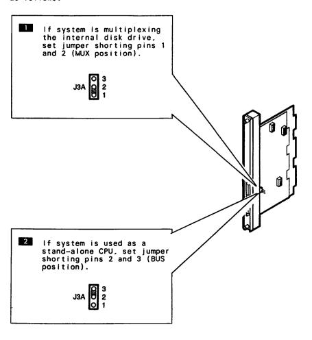
B.6.3.3 Multiplexing CS-D, CS/386-D Internal Disk Drives (Sheet 1 of 3)
