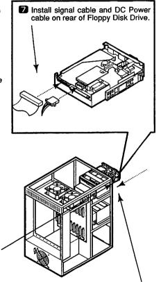
B Push Floppy Disk Drive into cabinet and mounting brackets will lock into position.
