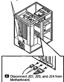
Remove remaining two (2) Phillips-Head Screws attaching SPS-255 Power Supply to CS-D Chassis floor plate.
