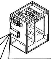
Disconnect DC Power cable connected to rear of Winchester Disk Drive.
