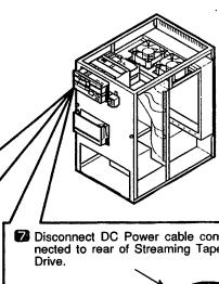
Disconnect DC Power cable connected to rear of Streaming Tape
