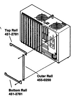
Position the outer rail (455-0290) for the CPU cover on the chassis lip between the top and bottom CPU cover rails, as shown.
