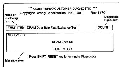
4 Errors will be displayed in the message field. All failures should be resolved. Test times with 32M memory along with the most likely failures would be:
