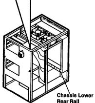
6 Slide motherboard up to free the mounting rails from the lip that supports them and remove it from the chassis.
