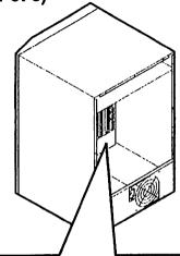
5 Disconnect power cables from motherboard connectors J22, J23, and J24.
