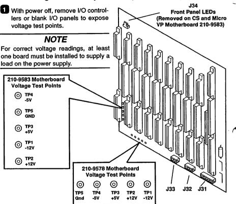
2 Be careful not to short out against any of the I/O boards. Using a voltmeter with straight pointed leads, measure each voltage.
