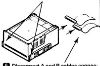
6 Disconnect A and B cables connected to rear of Winchester Disk Drive.
