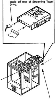
Install signal cable and DC Power
