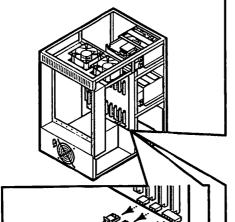
6 Remove DC Power harness plugged into connectors J22, J23, and J24 mounted on lower right corner of Motherboard.
