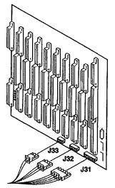
Remove all retaining screws securing motherboard to chassis. Remove motherboard.
