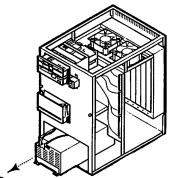
Remove SPS-255 Power Supply from front of CS-D Cabinet.
