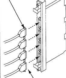
3 Note location and remove each interface cable connector.
