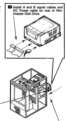
Push Winchester Disk Drive into cabinet and mounting brackets will lock into position.
