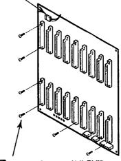
Remove fourteen (14) Phillips-Head Screws fastening Motherboard to CS-D Chassis.
