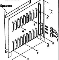
6 Remove eight screws securing motherboard to chassis. Remove motherboard. Note: There may be spacers behind the motherboard to raise it. These will not be used with the Turbo motherboard.
