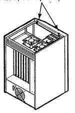
Slide Front Cover upwards, and lift away from CS-D cabinet.
