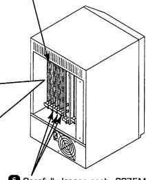
6 Carefully loosen each 2275MUXE Board (up to 3). Do not remove.
