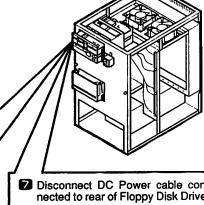
Disconnect DC Power cable connected to rear of Floppy Disk Drive.
