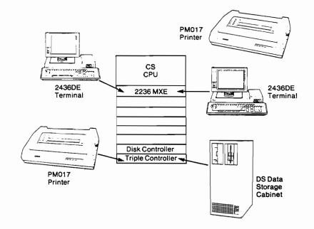
Figure 1-1. Typical CS Configuration
