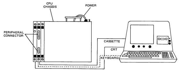
A unique feature of the Model 2220 is the cassette drive/keyboard controller board. This board accepts both the Model 2220 Single Tape Cassette Drive connector and the Model 2220 Upper/Lowercase Alphanumeric/BASIC Keyboard connector, thereby making available an additional I/O slot for any one of Wang's full line of peripheral devices.
